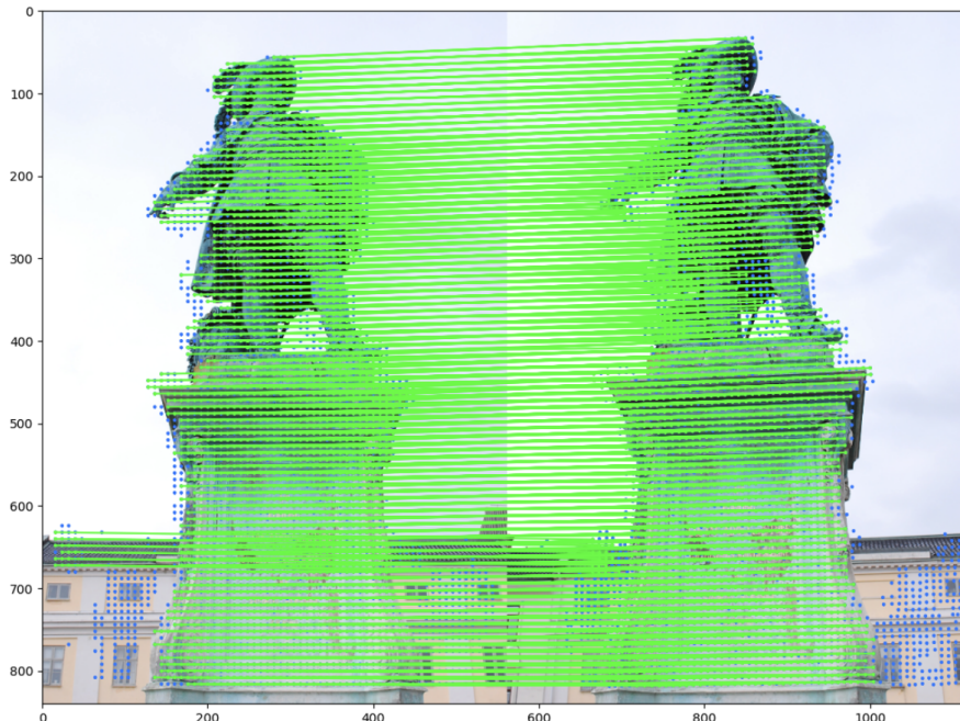
LOFTR Feature Detection Algorithm Results on Dataset.
